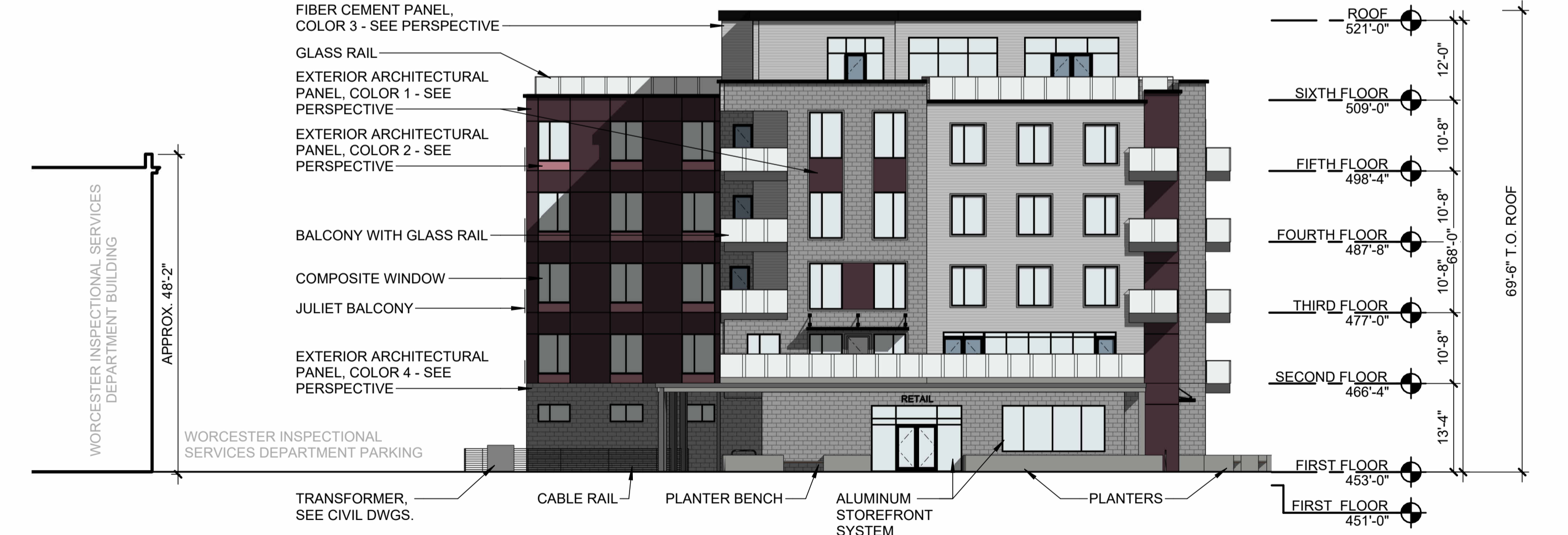
EAST ELEVATION - MEADE STREET 1 SCALE: 1/16" = 1'-0"
